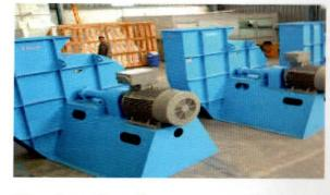
Steel casing for process fan, cooler and non standard parts
